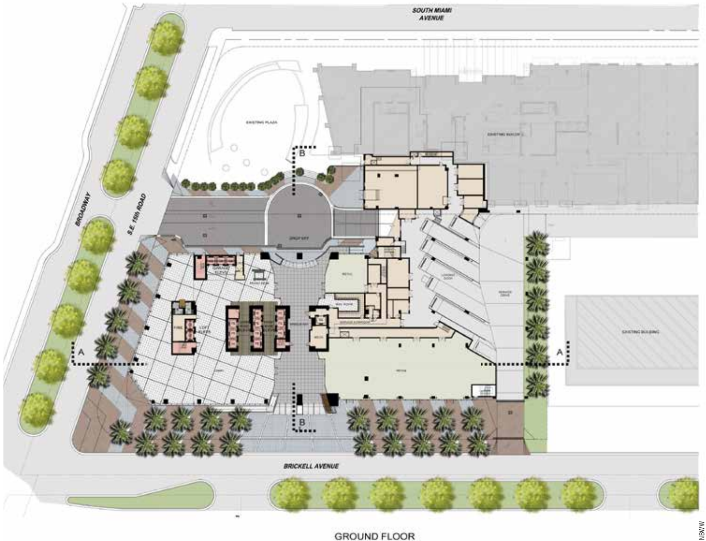
The ground-floor plan, showing the office lobby on the left, retail space and loading docks on the right, the breezeway through the middle, and the auto entrance drive with access to the parking garage near the top of the plan. A bank now occupies the corner on the left within the lobby.
