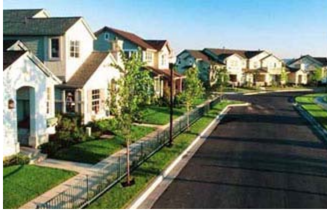
Residential streets are kept as narrow as possible, and intersections are "bulbed" to help calm traffic.
