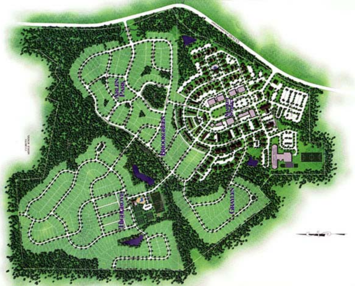
The site plan for Southern Village demonstrates its neotraditional features, including interconnected streets, a village center, and integrated open space.
